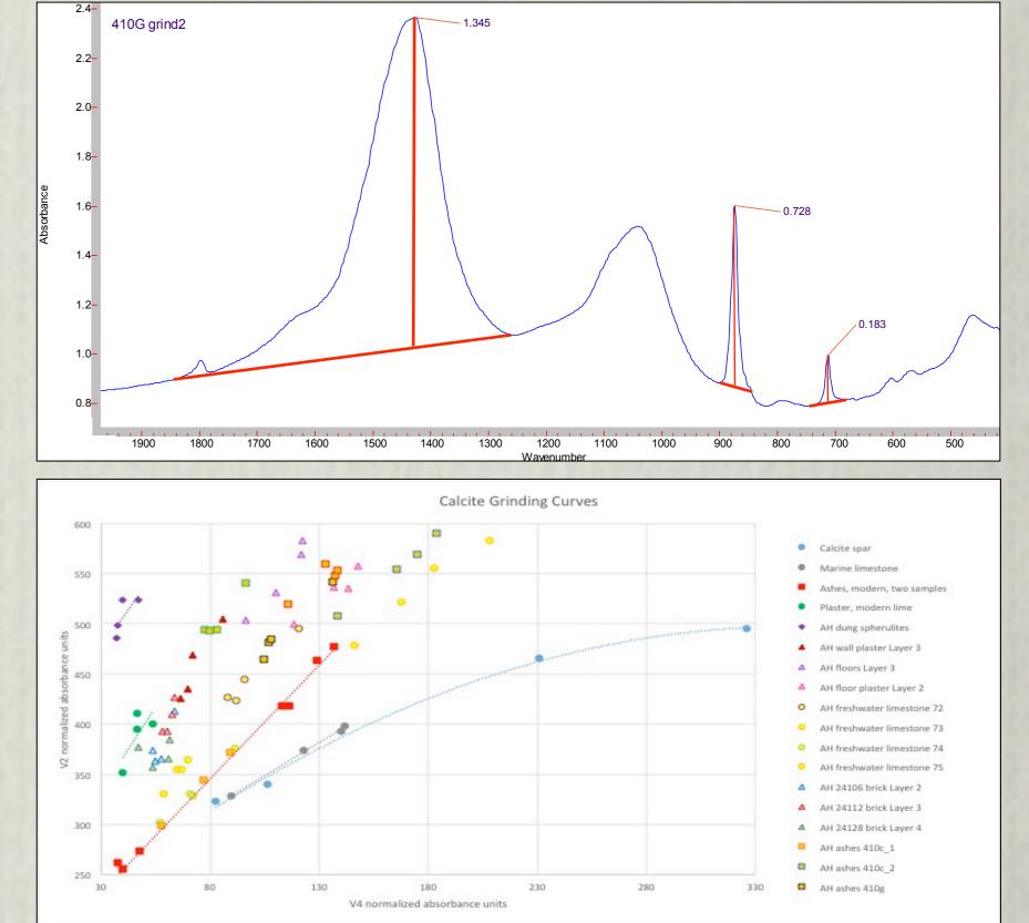
Analysis of calcite using grinding curves has been reported as an approach to distinguishing between calcites of pyrogenic origin (ash and lime plaster) and geogenic origin (Regev. et al. 2009). We produced a plot of calcite grinding curves using locally available calcareous materials, modern references, and construction materials from the site.
