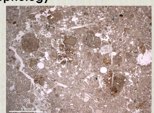
Mortar with vegetal voids, vesicles and aggregates derived from a soil, PPL.
